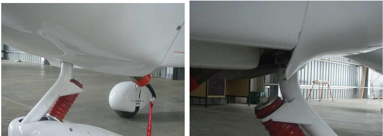
Figure 55: Lip to aid cooling as installed on a Jabiru.
