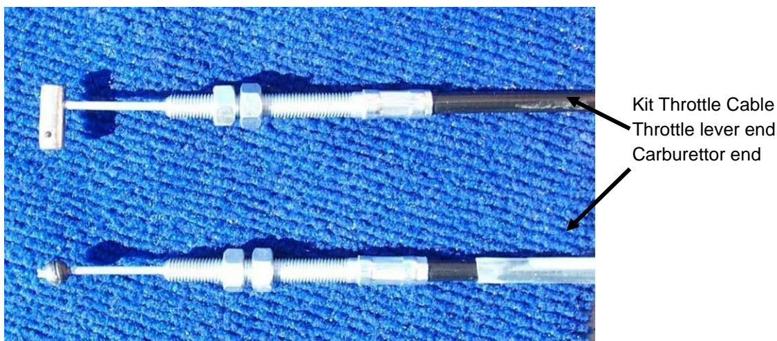
Figure 2: Throttle cable connections.
