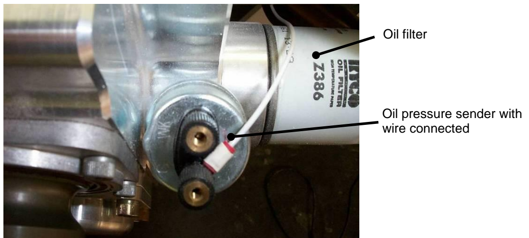
Figure 21. Oil Pressure Sender
