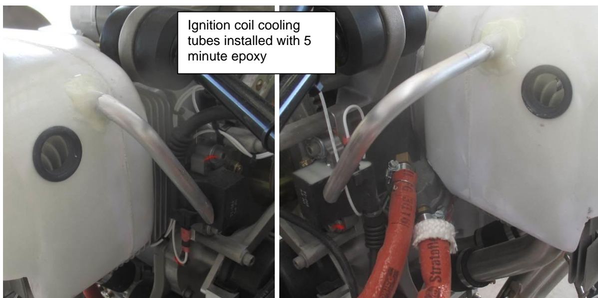
Figure 50: Ignition coil cooling tubes
