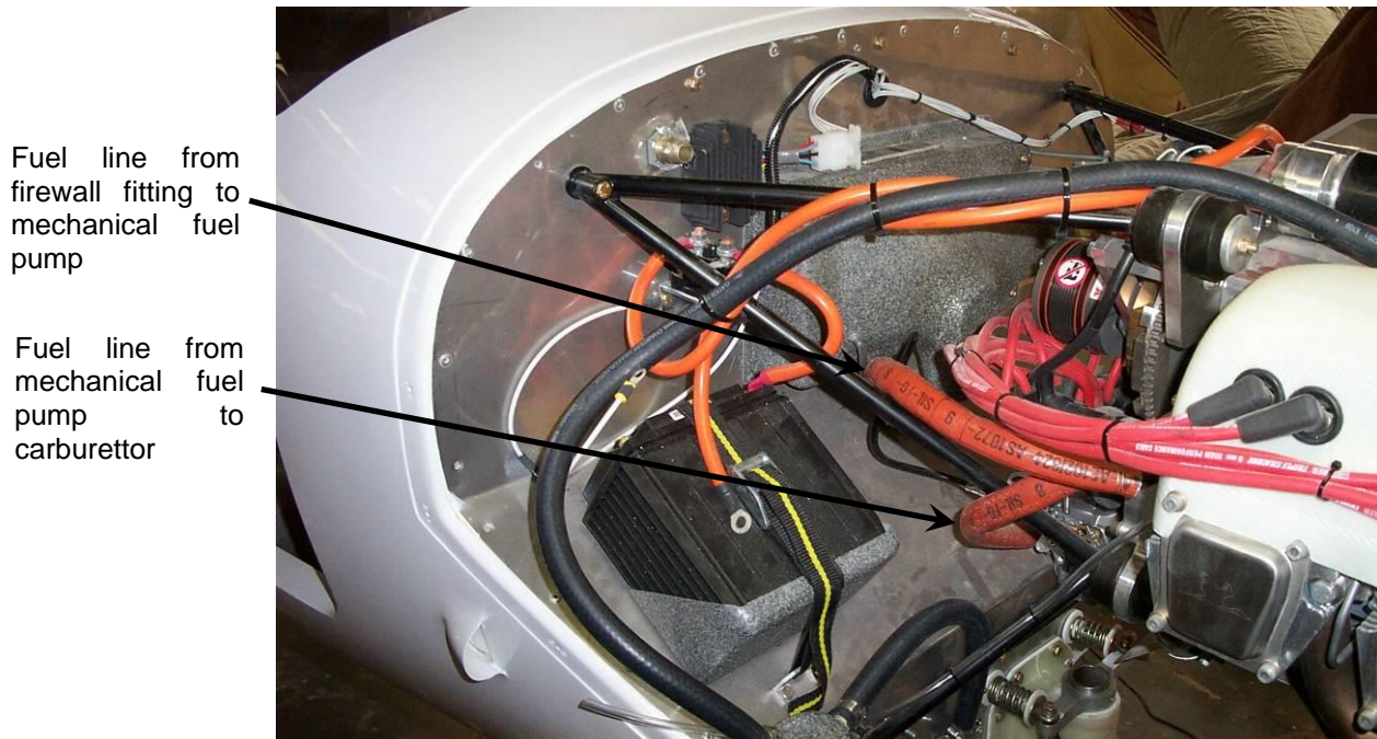
Figure 41. Fuel Connections General
