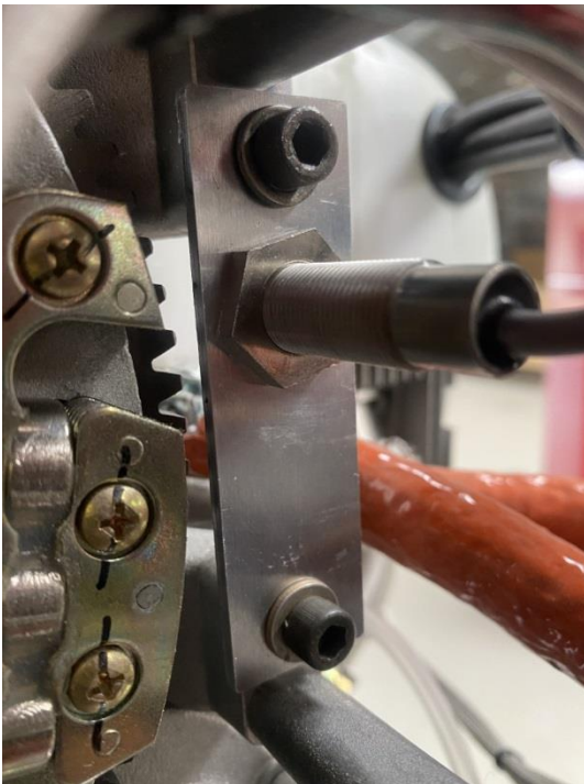
Figure 17: Hall effect sender mounting location on 3300 engine.
