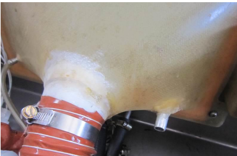
Figure 29: Balance tube connection on airbox.
