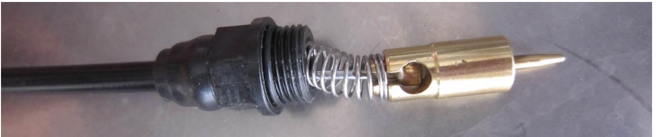
Figure 6: Choke cable end assembled.
