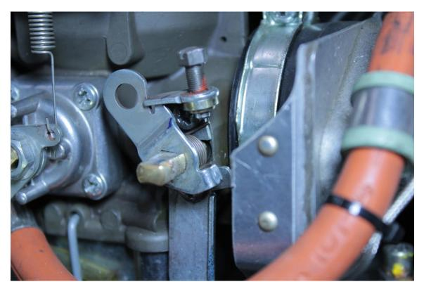
FIGURE 1: SPRING INSTALLATION (THROTTLE ARM NOT INSTALLED)
