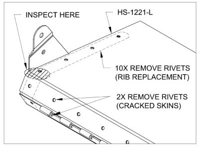
FIGURE 1: INSPECT FOR CRACKS
