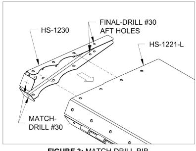
FIGURE 3: MATCH-DRILL RIB
