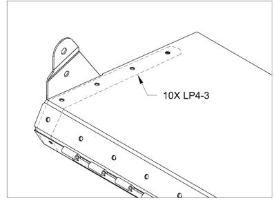
FIGURE 5: INSTALL INBD RIB
