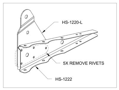
FIGURE 2: REMOVE HORN FROM RIB
