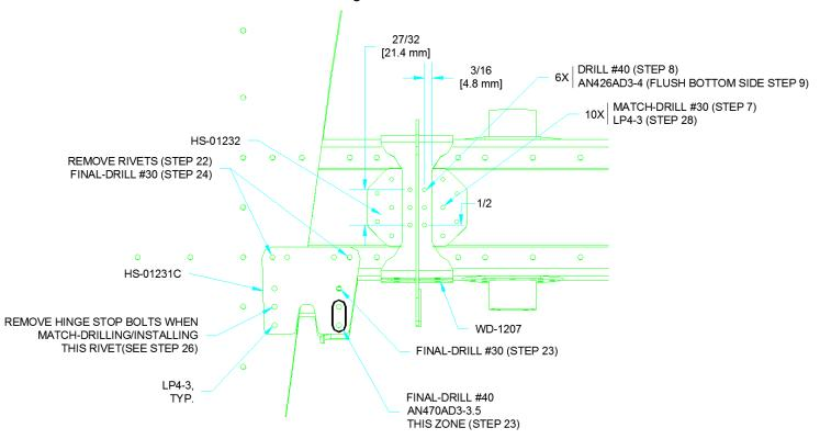
FIGURE 8: INSTALLING THE STABILATOR HINGE GUSSETS
