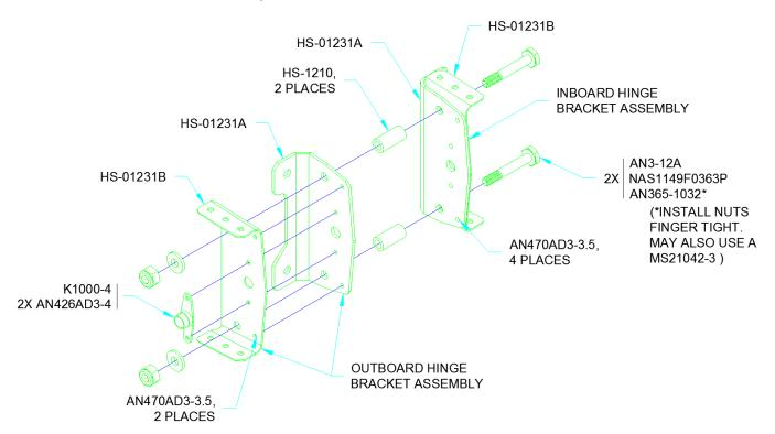
FIGURE 6: ASSEMBLING THE INBOARD AND OUTBOARD HINGE BRACKET ASSEMBLIES
