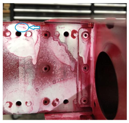
FIGURE 1: DYE PENETRANT TEST CRACK DETECTION
