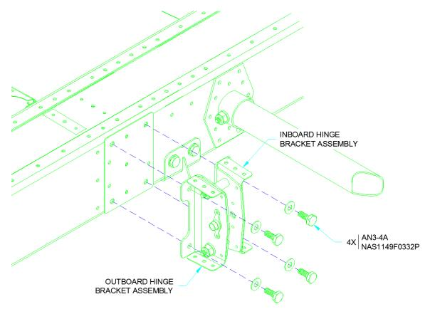
FIGURE 7: ATTACHING THE HINGE BRACKET ASSEMBLIES TO THE MAIN SPAR
