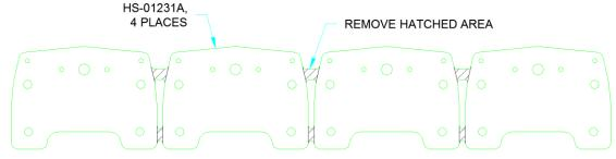
FIGURE 5: SEPARATING THE STABILATOR HINGE ANGLE (SHOWN FLAT)
