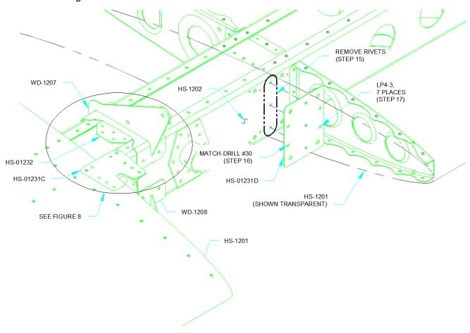
FIGURE 4: ADDING THE STABILATOR HINGE DOUBLERS
