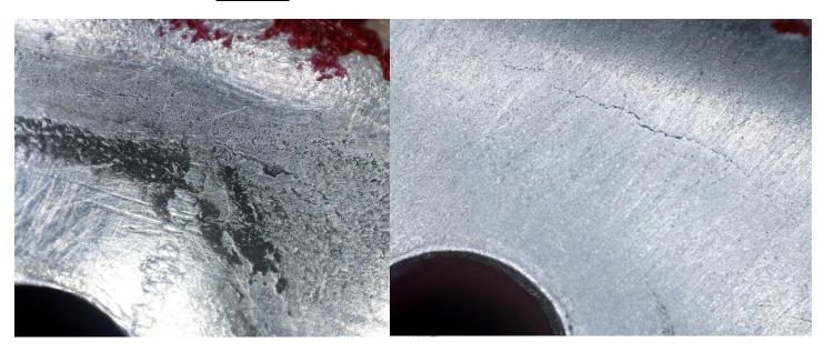
FIGURE 2: CRACK AFTER REMOVAL OF DYE PENETRANT
