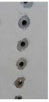
FIGURE 3: REMOVED RIVET HEAD PAINT BUILDUP
