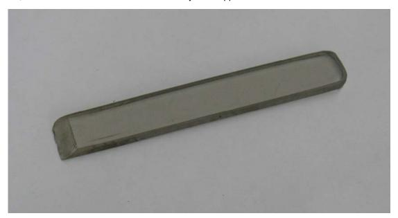
FIGURE 4: SEALANT REMOVAL TOOL
