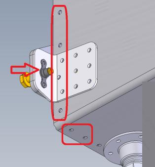
FIGURE 2: REMOVING INBOARD RIVETS AND NUTPLATES
