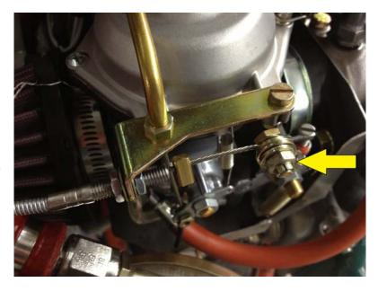
FIGURE 2: MS21045-3 INSTALLED
