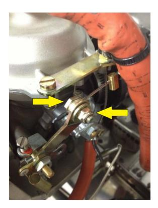
**FIGURE 1:** VA-219 INSTALLED WITH INCORRECT M5 ROTAX NUT
