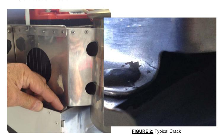
FIGURE 1: Crack Location
