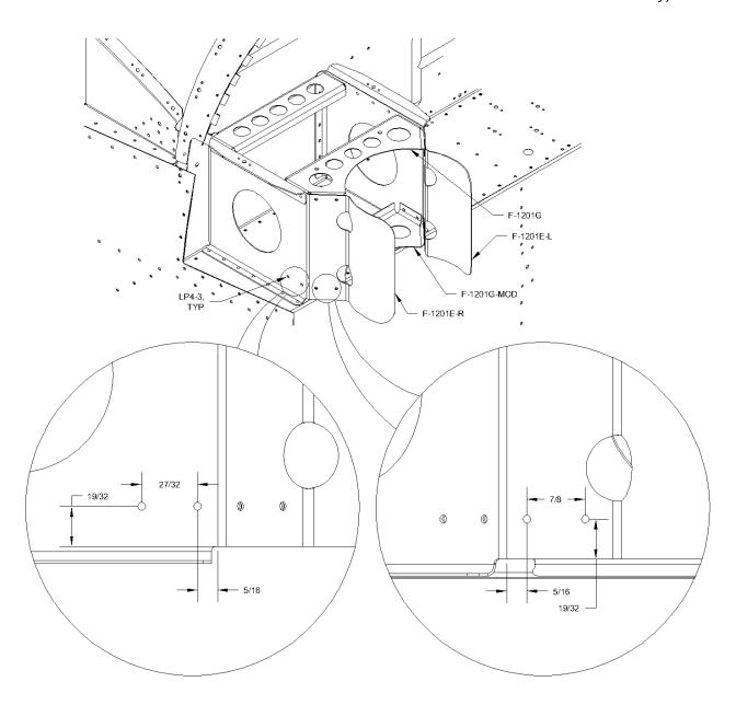
FIGURE 4: Rib Installation
