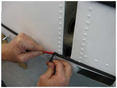
FIGURE 4: REMOVING THE SEAL STRIP
