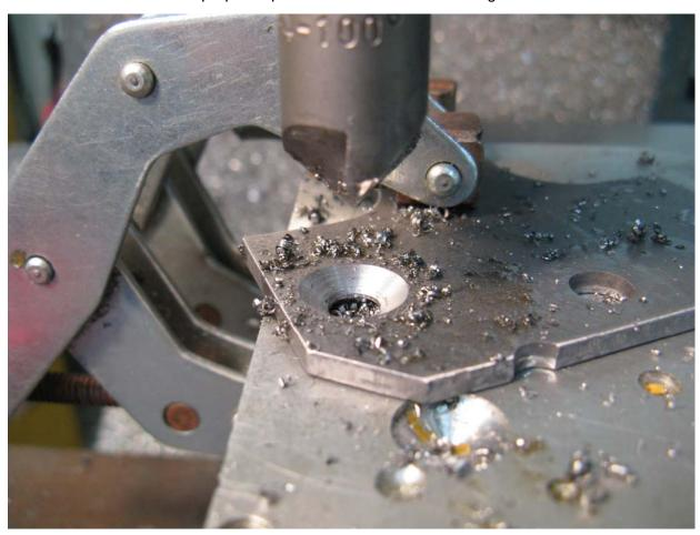
FIGURE 19: MACHINE-COUNTERSINKING
