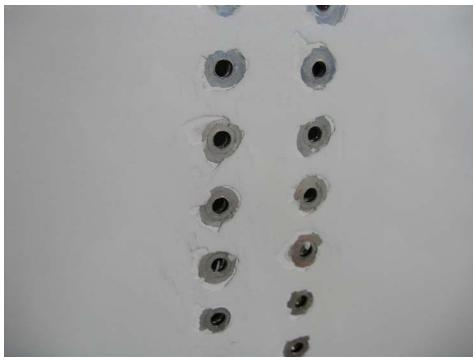
FIGURE 8: REMOVED RIVET HEAD PAINT BUILDUP
